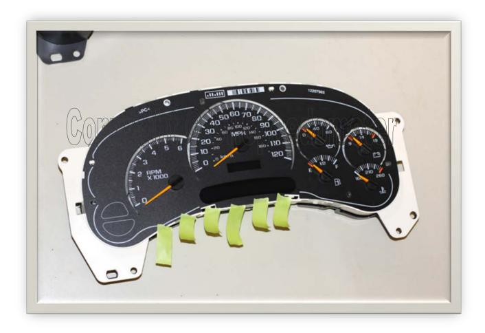
Rotate each needle counter clockwise until they come to their stopping point. Stick the tape to the gauge face plate directly below the needles. Look straight down on each gauge and make a mark directly in line with the tip of the needles. These marks will give you a reference point to set your needles back exactly where they were originally after you replace the stepper motors, ensuring accurate readings upon reinstallation.
