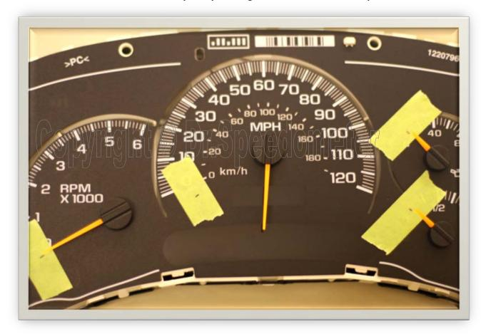
Now slide the pry tool under the gauge base being sure the fork tines are going around either side of the shaft. Next, pry upwards on the gauge base by pressing down on the pry tool. Be careful not to scratch your face plate. Pry firmly but slowly and the gauge will slide upwards and off the shaft. Move on to each gauge using the same technique.
