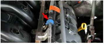
29. Unplug the eight (8) fuel injector connections (driver side shown) by pushing down on the tab and pulling plug out of injector.
