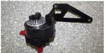
78. Locate the two (2) holes on the driver side air box support and install intercooler pump and bracket assembly using the M8 x 20mm bolt and Nut located in bag #3. **NOTE:** The bolt on the left can be loosely installed at this time. The intercooler relay ground wire will connect to this point later.
