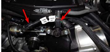
C) Connect the relay harness to the previously installed intercooler water pump and fasten the ground strap to the pump bracket.
