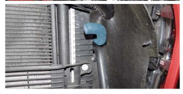
83. Install water pump to LTR hose using the supplied pinch clamps in bag #3 and route through the radiator shroud as shown.
