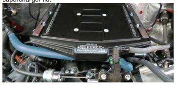
74. Remove the EVAP solenoid from the factory manifold using an 8mm socket. Install the EVAP solenoid to the supercharger manifold using two (2) M6 x 25mm bolts in Bag # 1. Reconnect the Evap line to the solenoid.
