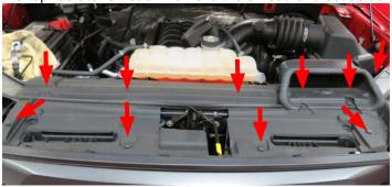
16. Using an 8mm socket, remove four (4) bolts securing the grille.
