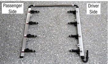
68. Apply O-ring lube to both ends of the supplied fuel injectors, then install them into the supplied fuel rails, oriented so the electrical connectors will face away from the supercharger.
