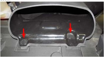
109. Secure the head light fascia by carefully pushing it back into place and reinstall the factory push pins.
