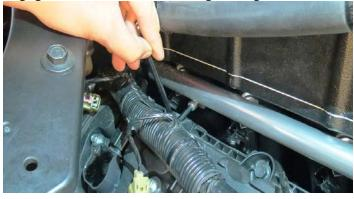
71. Reconnect the injector connectors to the appropriate fuel injectors. **WARNING: Never attempt to rotate the injectors**.
