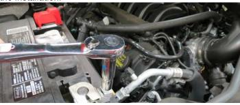
14. Drain the coolant by loosening the petcock located on the driver side of the radiator. *TIP:* Placing a hose onto the drain spout will reduce potential coolant spillage.
