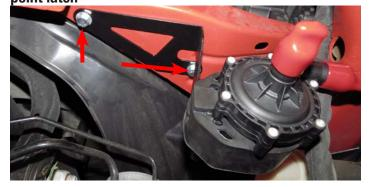
79. Remove the indicated strut tower nut and install intercooler reservoir bracket over stud. Loosely tighten the strut tower nut. Using the supplied M8 x 20mm bolt, washers and nut located in bag #3, fasten the bracket to the hole on the back of the control arm mount. Install intercooler overflow tank on bracket using the supplied M6 x 10mm bolts and alight bracket so tank is sitting upright. Tighten all hardware. **Do not overtighten bolts securing tank to bracket.**
