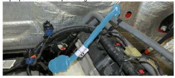
63. Remove the O-ring manifold gaskets from the factory manifold and install them onto the supercharger runners. Apply a small amount of O-ring lubricant to the exposed area of the gaskets. This will help prevent tears during installation of the supercharger .
