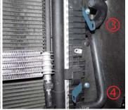
90. Using the measurements below, insert the plastic ties through the LTR fins in these locations from back to front. **DO NOT DRILL. Press in by hand ONLY.**
