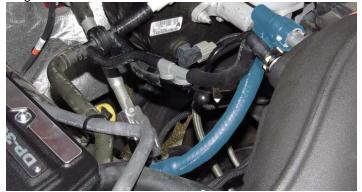
105. Verify that the coolant petcock is closed, then refill the coolant system. Use of a vacuum filler is recommended.
