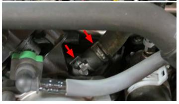
24. Disconnect the evap line from the purge valve by squeezing the green clip together at the bottom and lifting the tab up. Disconnect purge valve harness by pushing down the black tab and pulling plug out.
