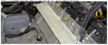
37. Tape up the four (4) IMRC harness plugs at the plug ends and secure plugs to the main harness out of the way. These will not be reused.
