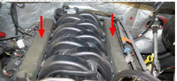
28. With the vehicle **COMPLETELY** cooled. Put rags under the fuel rail fitting and remove the fuel line from the rail by pulling the blue locking tab up. Cap off the fuel rail and fuel line with appropriate cap and plug to prevent spillage. Clean up and spilt fuel before proceeding.
