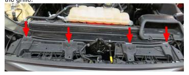
17. Using a panel puller, remove two (2) push pins on both sides of the truck holding the head light fascia in place. Carefully pull the front fascia forward on each side until the clips disengage and the lower grille bolts are exposed. Remove lower grille bolts using an 8mm socket and extension.
