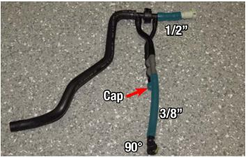
Install the new brake booster hose assembly using the factory clamps to secure the rubber line to the supercharger fitting. Push the two (2) remaining connectors onto their prospective fittings to lock them in place.
