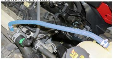
59. Using a panel removal tool, remove the engine harness from both valve covers. Using wire cutters, carefully cut harness retaining pins from the harness and discard.
