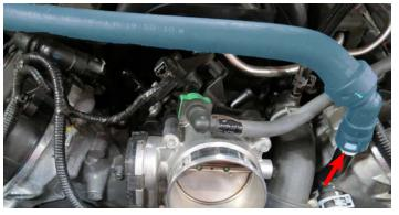
34. Lift the intake manifold and rotate counterclockwise as shown below. Locate the driver side IMRC position sensor harness and disconnect by pulling out the red locking tab, pushing down on the plug's clip and pulling the plug out. At this time, disconnect the MAP sensor harness located to the right of the driver side IMRC sensor. **See step #35 for plug locations.**
