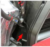
19. Unplug grille shutter control and ambient temp sensor located in front of the hood latch. Using a panel puller, remove harness from grille. Remove grille by lifting up and out and set aside.
