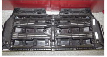
108. Reinstall the grille and radiator cover using the factory hardware and the two, new push pins that secure the air scoop as shows below. Be sure to reconnect the grill shutter harness even though this feature is no longer used.
