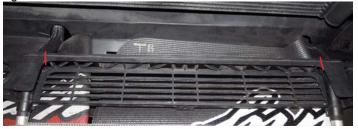
89. Install the LTR brackets by first removing the plastic push pins in locations #1, #3 and #4. Orient the brackets as shown below and secure with the supplied hardware. Leave hardware slightly loose for adjustment later. Note: The brackets should be mounted under the rubber radiator shroud. The bolt and washer will hold the shroud and bracket in place. All hardware is located in bag #3.
