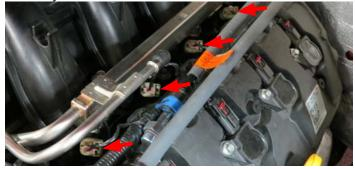
30. Using a 10mm socket, remove four (4) fuel rail bolts (driver side shown). Firmly and evenly lift up on fuel rail from both sides and remove from intake manifold.
