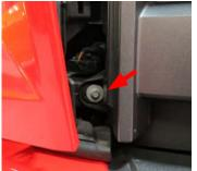
18. Remove six (6) push pins securing the flexible radiator shroud to the grille (3 pins per side). Tip: The two (2) lower pins (not pictured) can be removed by hand carefully if tool is not accessible.
