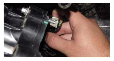
35. Rotate the intake manifold clockwise to gain access to the passenger side IMRC sensor harness and disconnect as described above. Make sure the plastic push pins are disconnected from the back of the manifold in the locations shown below (red arrows).
