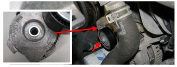
39. Using a 3/8" breaker bar or equivalent, release the tension from the secondary A/C drive tensioner and remove the A/C drive belt and discard.
