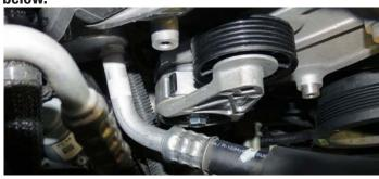
56. Install two (2) idler pulleys, one (1) 76mm and one (1) 70mm, with two (2) M8 x 20mm bolts and washers from bag #2. The smaller 70mm pulley should be installed on the uppermost boss on the tensioner bracket. Torque both idler pulley bolts to 22 ft-lbs.
