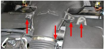
31. Lift the airbox and resonator tube off the locator pins and remove it and the air inlet tube as an assembly.
