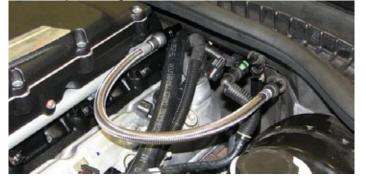
204. Connect fuel injector electrical connectors.
