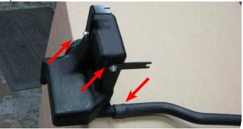
177. Use a 10mm socket to loosen rear hood hold down latch bolt on passenger side fender.
