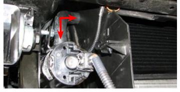
170. Lower the heat exchanger hose assembly along the driver side of the radiator shroud.
