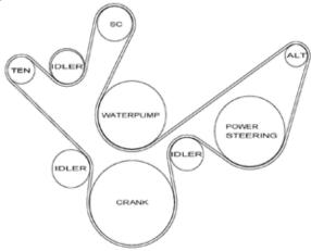
217. Use a breaker bar and a 16mm socket to push the tensioner enough to get the belt on, then double check the routing.
