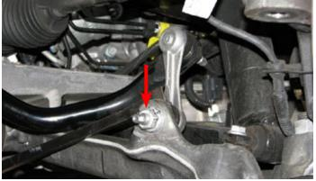
80. Use a 13mm socket to remove the four bolts retaining the stabilizer brackets.
