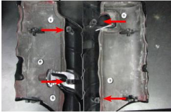
209. Remove the grommets from the stock coil covers.
