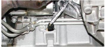
96. Use a 10mm socket to remove the starter support bracket bolt.
