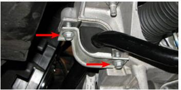
81. Use a 10mm socket to remove the two nuts retaining the brake pressure modulator valve.
