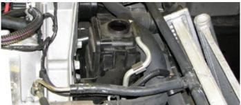
73. Disconnect the alternator electrical connector.
