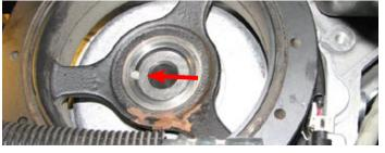
106. Install the supplied GM crank bolt into the crank and torque it to 37 ft-lbs, then rotate it an additional 140°
