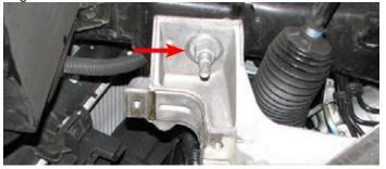
86. Disconnect the ride height sensor electrical connector from each side, if equipped.
