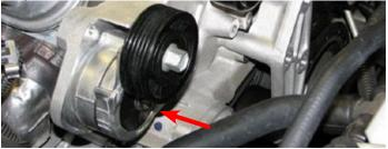
147. Use a 12mm socket and a 20mm bolt supplied in Bag #1 to mount the EVAP purge solenoid on the back of the new tensioner bracket.
