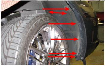
21. Pull back the inner fender well to access the two bumper studs on each side. Use a 10mm deep socket to remove the nuts.
