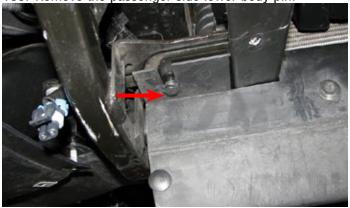
160. Use a 10mm socket to loosely install the water pump bracket using the stock horn bracket bolt on top and the bolt supplied in Bag #3 on the bottom.
