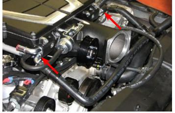
202. Attach one end of the supplied PCV hose to the  $90^{\circ}$  fitting below the air inlet on the supercharger. Route the other end of the PCV hose to the tube extending from the valley plate and attach
