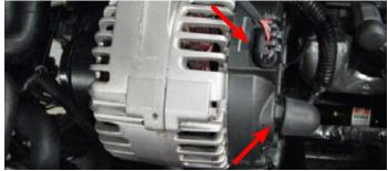
74. Use a 13mm socket to remove alternator power wire.
