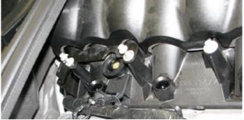
44. Use a 10mm socket to remove the seven remaining manifold bolts (out of ten).
