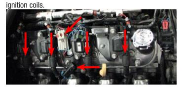
37. Use a 10mm socket to remove the five bolts retaining the coil bracket on each valve cover then remove both coil bracket assemblies.
