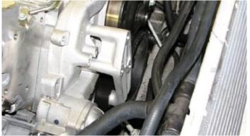
143. Use a 15mm socket and the two stock bolts to mount the new tensioner bracket onto the water pump then torque them to 37 ft-lbs.
