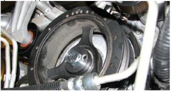
103. Use a 24 mm socket to install the supplied bolt and reamer guide to the end of the crank.
