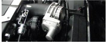
219. Connect ETC harness to the throttle body motor.
