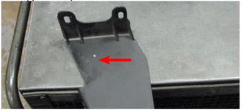
164. Use a 10mm socket and the four stock bolts to reinstall the upper radiator shroud then attach the relay off the supplied water pump wire harness to the upper radiator shroud using the supplied body pin. Open and close the hood to verify the relay clears the hood strut.
