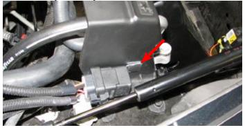
165. Route the intercooler water pump wire harness extending from the relay down to the intercooler water pump and plug in the connector.
