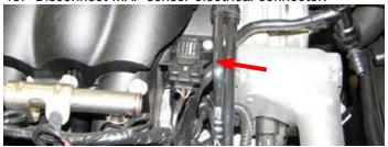
47. Disconnect the vacuum hose from the brake booster fitting; it will be removed with the manifold.
