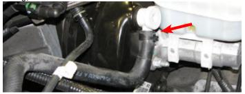
48. Disconnect and remove the two EVAP tubes located at the front of the manifold.
