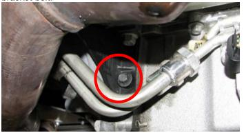
97. Use a 13mm socket to remove the two starter bolts.
