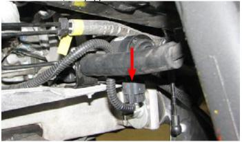
87. Use a 10mm socket to remove the driver side brake line bracket bolt.
