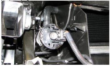
166. Plug the male connector on the T-segment of the harness into the EVAP solenoid then plug the factory EVAP connector into the female connector on the T-segment.
