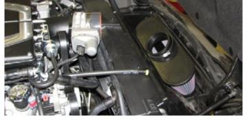
225. Use a T20 Torx driver to remove the MAF sensor from the stock airbox.
