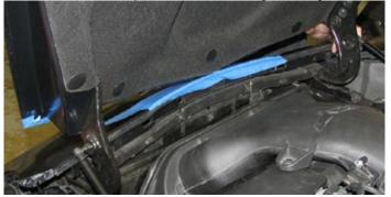
27. The sides of the fascia can be pulled away from the clips holding it in place, then down off the studs. The center section must be pulled up and over the nose section, and the whole assembly pulled straight off and set aside.
