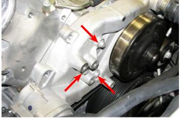
142. Use a 6mm Allen tool and the three 90mm bolts supplied in Bag #1 to install the lower idler bracket on the water pump then torque them to 18 ft-lbs.
