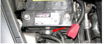
17. Remove the battery and set it to aside.
