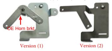
161. **NOTE:** This step only applies to customers who received version (1) of the water pump brackets. Install the supplied stand-off and lock nut onto the OE horn bracket. Proceed by mounting that assembly, with the supplied M6 x 10mm bolt, to the water pump bracket as shown below.
