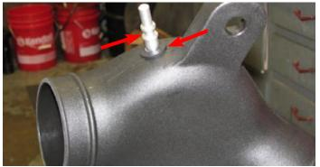
223. Install the hose barb supplied in Bag #5 into the new air inlet tube.
