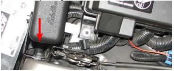
178. Install intercooler reservoir by working molded hose down along the passenger side of the radiator to the water pump inlet and secure the hose on the pump fitting with a hose clamp supplied in Bag #2.
