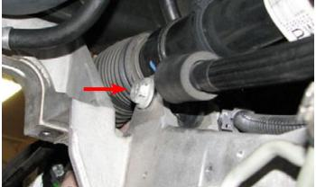
91. Remove the plastic clamp holding the power steering lines to the steering rack.
