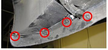
24. Remove the five 7mm and two 10mm nuts retaining the fascia from below.
