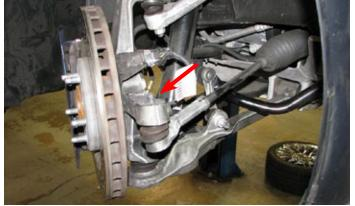
78. Use GM Ball Joint Separator #J 42188 to separate the steering knuckle from the tie rod ball stud then remove the tool and the nut. Use this procedure for both sides.
