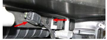
69. Disconnect the ambient air temperature sensor and remove the sensor clipped to passenger side of shroud.
