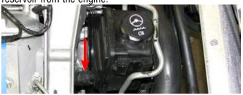
149. Slide the old bracket off the reservoir then install the supplied bracket using a 15mm socket and the stock bolts. Slide the power steering reservoir onto the new bracket and reattach the lower reservoir to pump hose.
