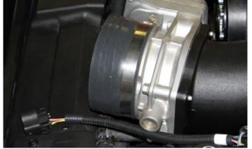
222. Install the grommet supplied in Bag #5 into the new air inlet tube.
