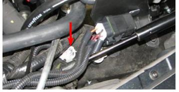
183. Reinstall the fender well fuse box bolt.
