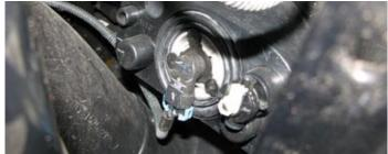
23. Remove the three screws and one body pin that retain each front valance.
