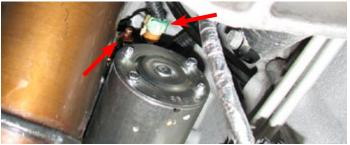
99. Remove and set the starter and bracket aside.
