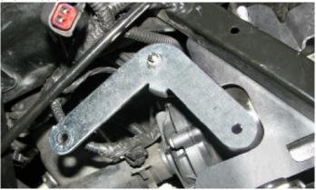
162. Re-install the horns using the OE nuts. Be sure to orient the horns so that there is slack in the horn's wiring harness. *Warning:* Do not mount the horns with the openings facing up, as they may accumulate condensation and cease working.
