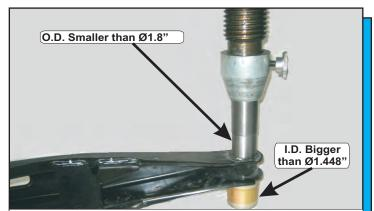
I.D. of rear lower control arm inner position is Ø1.448". Using a hydraulic press, properly support control arm and slowly push out the rubber bushing with bonded outer metal shell. Remove all sharp edges from I.D. Apply grease to all metal parts that will contact the new polyurethane bushings.
