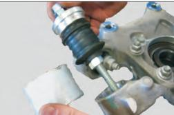
Refer to the shop manual for the safe removal of front and rear control arms, torque specs, and alignment of your vehicle. Removel of the factory bushings on the trailing arm, adjuster link & knuckle will all be the same. The bushings are not bonded & no metal shell to press out.
